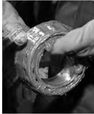
Fig. 23. Grease can easily be packed by hand.
