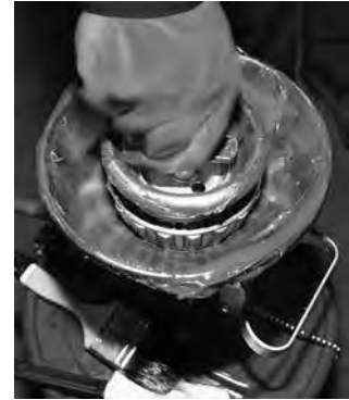
Fig. 24. Mechanical grease packer.
